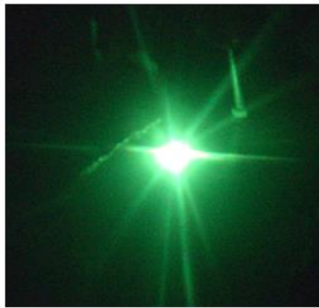
Figure 5. Arc in TIG welding without flux
