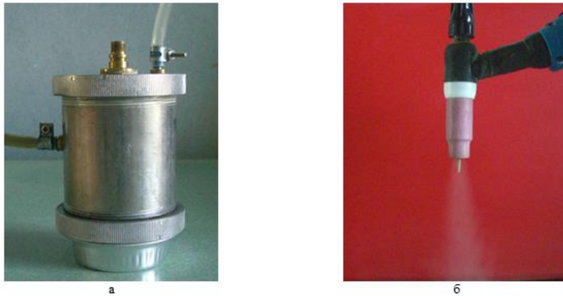
Fig. 2. The feeder for producing the gas-powder mixture (a) and the welding gun with gas-powder mixture (b).
