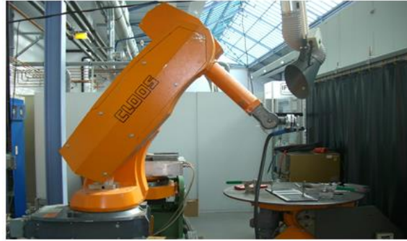
Fig. 4. Flux feeder, mounted on a welding robot
